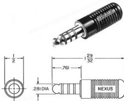
TP-101 (U-174/U, M9177/2-1) Four Conductor Telephone Plug Mates with NEXUS Series TJ-120 and TJ-102 jacks and jack TJ-101. One piece monel contacts integrally molded with glass filled nylon plastic.
