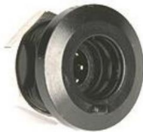
AJ-117PM Miniature Front Panel Mount Waterproof Jack Panel mount from front of panel, 7 conductor miniature waterproof jack, solder terminals, mates with all versions of the AP-117. Nut and lockwasher are included.
