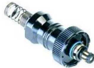
AP-117LR-AL Miniature Waterproof Plug W/Locking Ring Seven conductor, miniature waterproof plug with locking ring, wire strain relief and solder terminals, .250" max. cable diameter, mates with AJ-117LR-AL.
